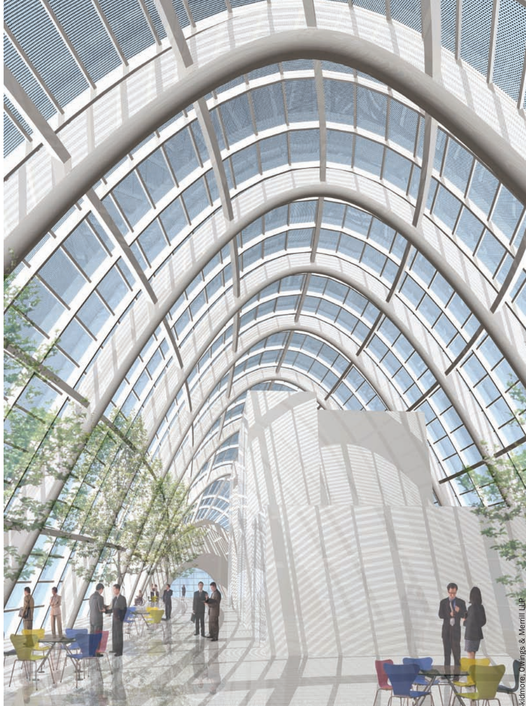
At the crown, PV technology is integrated into the façade glass.
