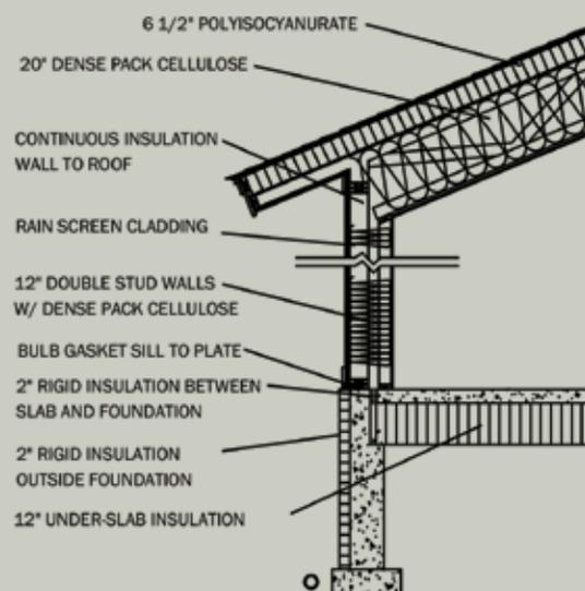
Insulation is continuous from under slab to wall to roof. The double-stud wall covers the slab-edge insulation. The parallel chord roof has top chord bearing allowing the interior non load-bearing stud to be attached to the end of the bottom chord of the roof truss forming a continuous insulation cavity. The rigid insulation on the roof keeps the dew point above the roof deck thus avoiding a cold surface where condensation could occur in winter.
